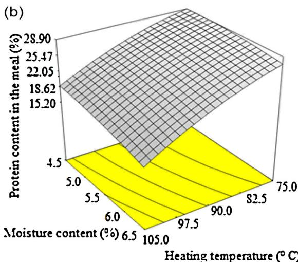
**Fig. 3.** (a) Linear design variation of protein content of the meal in diverse temperatures ( $\pm 1^\circ\text{C}$ ) and moisture contents of the output seeds of heating (%). (b) Response surface diagram in the protein content of the meals (%).
