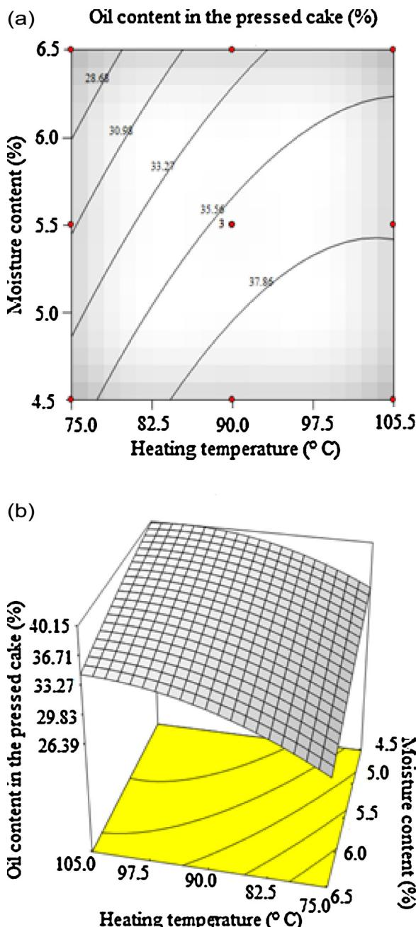
**Fig. 1.** (a) Linear design variation of oil content in the pressed cakes in diverse temperatures (°C) and moisture content of output seeds (%). (b) Response surface diagram of the oil content of the pressed cake (%).
