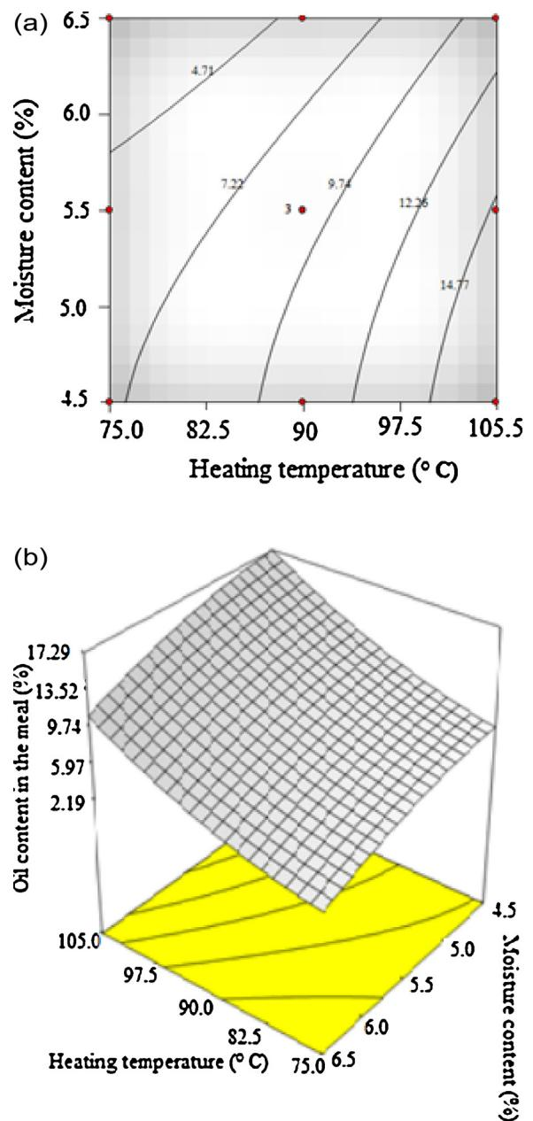
**Fig. 2.** (a) Linear design variation of oil content of the meal in diverse temperatures ( $\pm 1^{\circ}\text{C}$ ) and moisture content of the output seeds (%). (b) Response surface diagram of the oil content of the meal (%).
