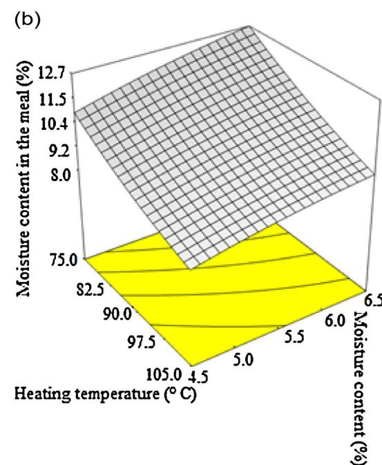
**Fig. 4.** (a) Linear design variation of moisture content of the meal in diverse temperatures ( $^\circ\text{C}$ ) and moisture contents of output seeds of heating (%). (b) Response surface diagram in moisture content of the meal (%).
