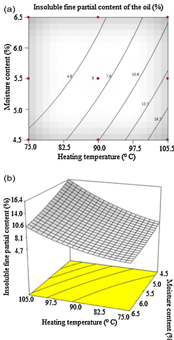
**Fig. 5.** (a) Linear design variations of insoluble fine partial content of extracted oil in diverse temperatures (°C) and moisture contents of output seeds of heating (%). (b) Response surface diagram for insoluble fine partial content of the extracted oil (%).
